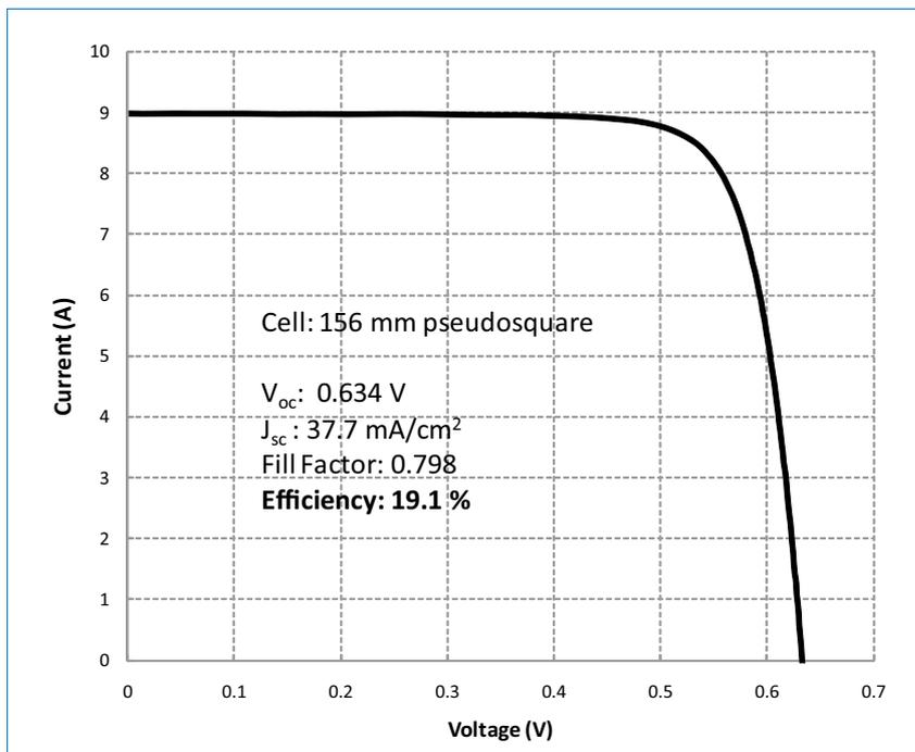
Figure 9. I-V curve of ion implanted cell ( $239\text{cm}^2$ ) with homogeneous emitter.
