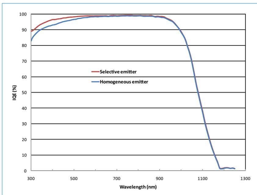
Figure 11. Measured IQE for cells having a homogeneous emitter and a selective emitter.
