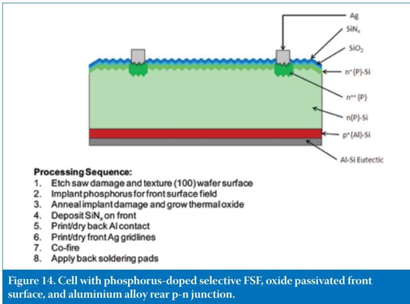
Figure 14. Cell with phosphorus-doped selective FSE, oxide passivated front surface, and aluminium alloy rear p-n junction.
