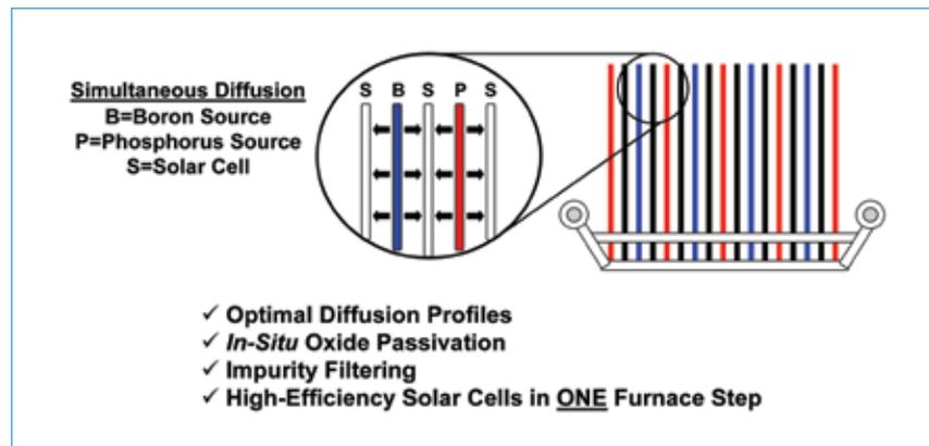
Figure 7. Original STAR process from UCEP, used to produce 20% cell efficiency (4cm<sup>2</sup> FZ), showing a solar cell wafer sandwiched between a boron source wafer and a phosphorus source wafer in a quartz boat.
