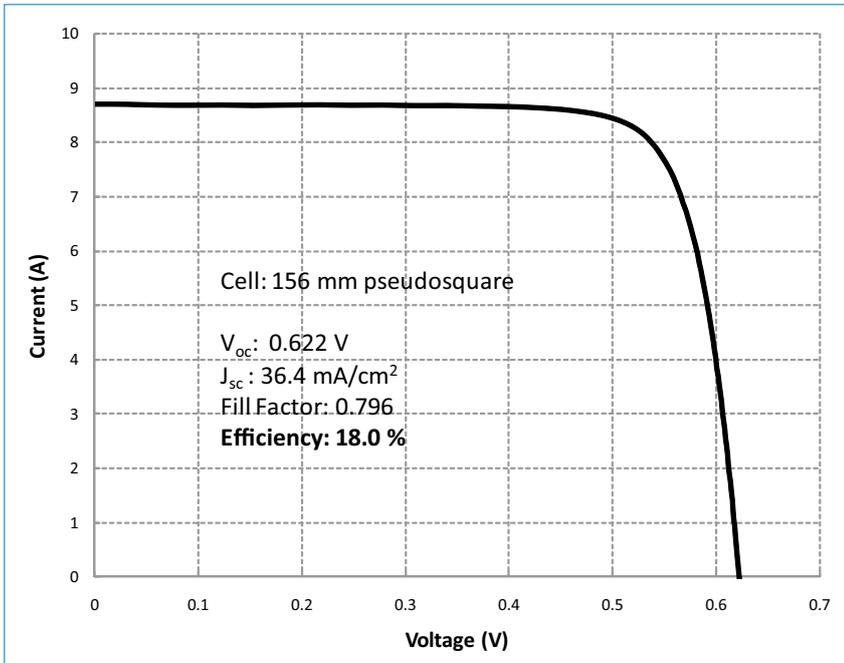
Figure 6. I-V curve for three-bus production cell (239cm<sup>2</sup>).
