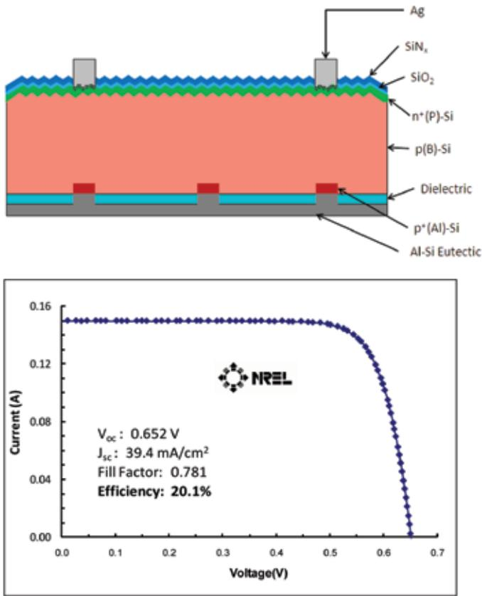
Figure 12. Structure of Delta-STAR cell (top) and corresponding current-voltage performance (4cm<sup>2</sup>FZ) (bottom).
