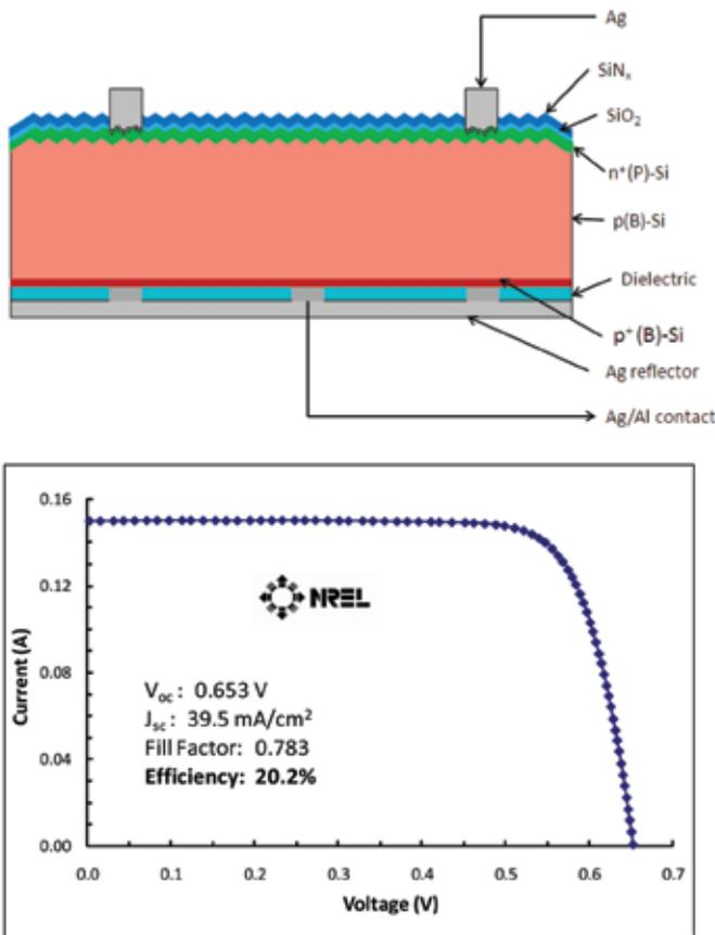
Figure 13. Structure of Beta-STAR cell (top) and corresponding current-voltage performance (4cm<sup>2</sup>FZ)(bottom).
