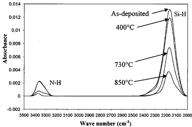
Fig. 2. FTIR spectrum of PECVD  $\text{SiN}_x$  films after post-deposition anneal.
