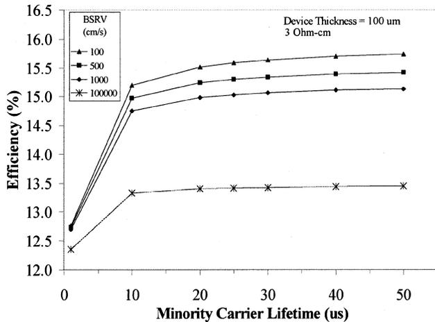
Fig. 1. PC1D simulation of the effect of  $\tau$  and BSRV on efficiency of string ribbon Si solar cells.
