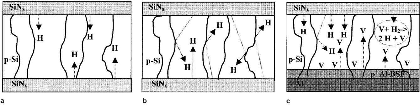
Fig. 5. A schematic representation of the three-step model for  $\text{SiN}_x$  induced defect passivation: (a) release of hydrogen during  $\text{SiN}_x$  anneal, (b) decrease in the retention probability of hydrogen at defects during high temperature  $\text{SiN}_x$  anneal, and (c) vacancy induced dissociation of molecular hydrogen and enhanced migration of atomic hydrogen.
