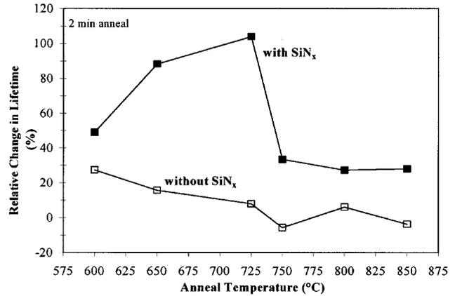
Fig. 3. Defect passivation from post-deposition anneal of PECVD  $\text{SiN}_x$ .
