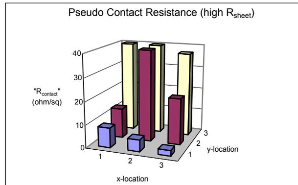
Fig. 3. High pseudo contact resistance map. Regions where “ $R_{\text{contact}}$ ” is high (approximately equal to the sheet resistance of the emitter layer) indicate almost no transfer of current from the emitter layer to the gridlines.
